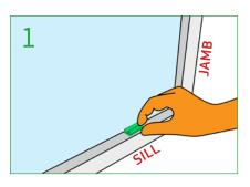
Fit glass panel to frame as required. Place DBC1 and GBC1 against the glass ensuring that they are in the correct orientation.
