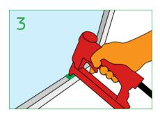
The clips can be fixed using staples, screws or pins. We recommend to use 2 x 80 series staples 12mm (or longer if preferred) per clip. With the air gun regulators set at approximately 4 bar. Ensure fixings do not protrude into clip channel and foul bead fitment.
