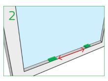
Ideal clip length is 35mm and 50mm (but longer lengths can be used if required). We recommend clips should be spaced at 150mm intervals. The more clips used, the stronger the fixing.
