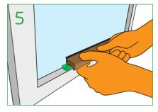
Offer DB1 bottom bead to slips. Angle in from one side to ease onto the clips.
