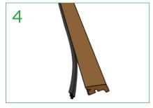
Measure and straight cross cut DB1 to meet the jambs. Then fit gasket to bead gasket slot in the profile. Ensure gasket allows a minimum gap of 2mm uncompressed.
