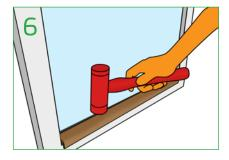
Once the bead is in the desired position on the clips, use a small glazing mallet to tap down into the final location. Check the bead is firmly located, it should not be able to be removed using your fingers.
