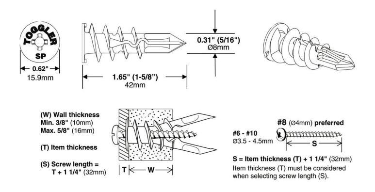
**Description** — SnapSkru Regular [SP] Self-drilling Drywall Anchor
