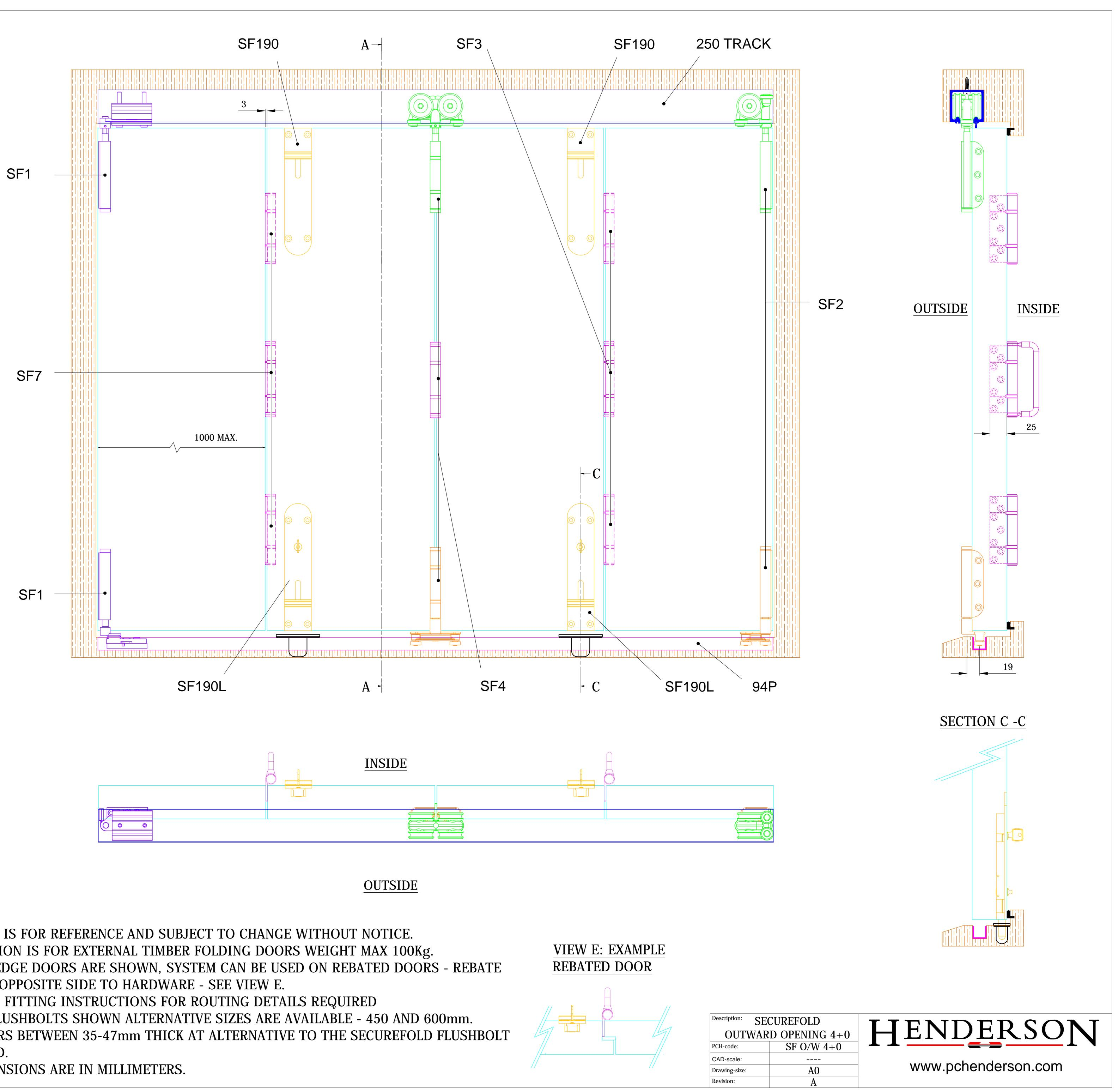
. DRAWING IS FOR REFERENCE AND SUBJECT TO CHANGE WITHOUT NOTICE. 2. APPLICATION IS FOR EXTERNAL TIMBER FOLDING DOORS WEIGHT MAX 100Kg. 3. SQUARE EDGE DOORS ARE SHOWN, SYSTEM CAN BE USED ON REBATED DOORS - REBATE SHOULD BE OPPOSITE SIDE TO HARDWARE - SEE VIEW E.
