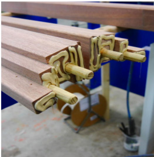
Figure 2: Applying adhesive in lines
