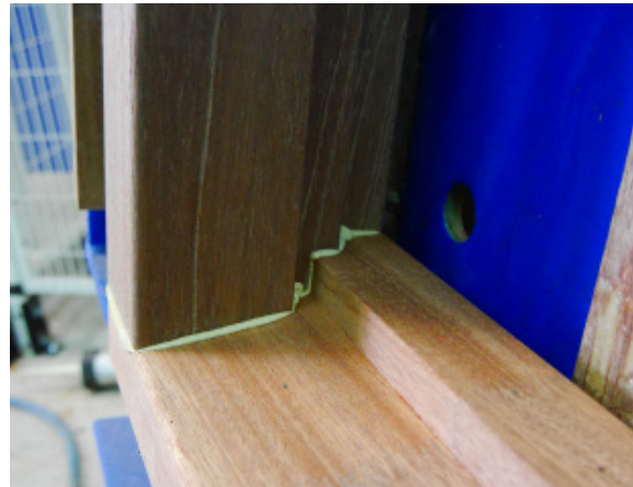
Figure 3: The adhesive is squeezed outwards.
