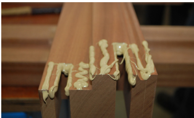
Figure 5: Applying adhesive rills to the threshold of a bridle joint
