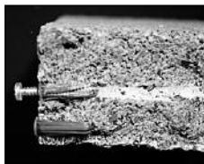
Plug anchor - NO extrusion & NO bonding
