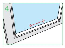
Pin beads every 150mm to 200mm securely to frame. Pin on end of each bead for extra security.
