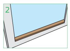
Check beads fit correctly in window frame.
