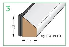
Apply 2.0 mm double sided glazing tape to glazing face of bead. Remove liner from glazing tape and apply beads to glazing into the frame.
