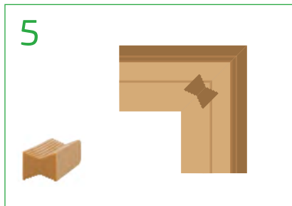
5 Join the pieces with butterfly joints to create the full cassette. (Hoffman W2, 6mm)
