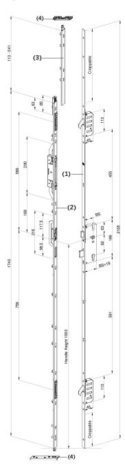
The FAB flushbolt keep rail is designed for French door systems with opposing eurogrooves
