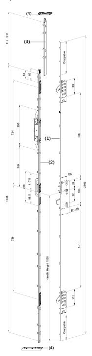
The FAB flushbolt keep rail is designed for French door systems with opposing eurogrooves
