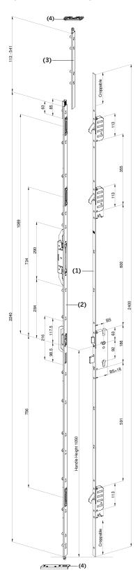
The FAB flushbolt keep rail is designed for French door systems with opposing eurogrooves
