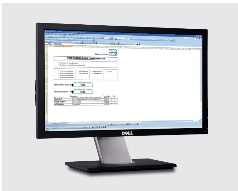
The Winkhaus FGTE Configurator is available on request and is used to identify parts based on input variables (i.e. Handle Height, Rebate Height, Backset, Handing, etc.). Excel 2003 or newer required.
